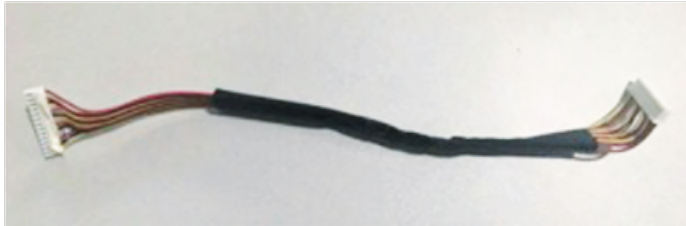
Parallel cable 2 (connect between the parallel card and the parallel connection board)
