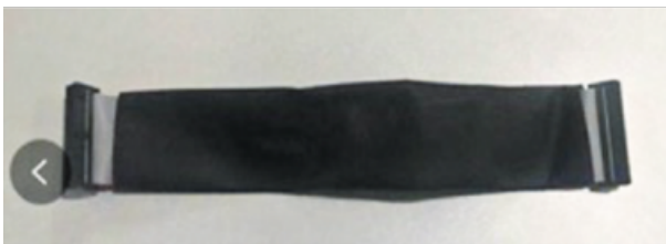
Parallel cable 1 (connect between the parallel card and the control logic board)
